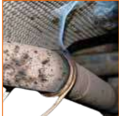
Loosening parts that are hard to access by using a special type of twisted wire
