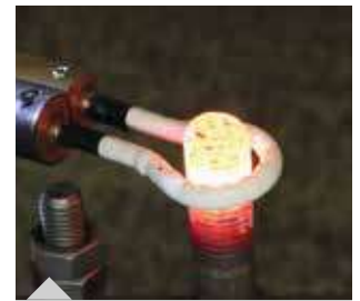
Heating a threaded bolt with the liquid-cooled coil
