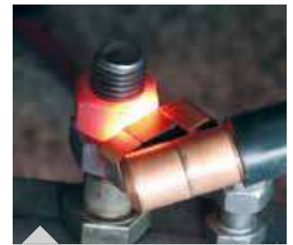
Heating a nut with the angled focusing coil
