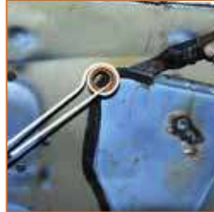
Easily removing small trim panels
