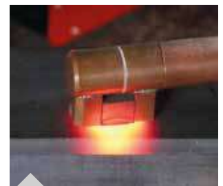
Heating a component with the straight focusing coil
